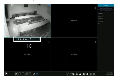
Click the preview window to show the tool bar as shown in area ①; right click the preview window to show the menu list (manually record on, instant playback, enable audio, snap, zoom in, PTZ control and camera info). The tool bar is introduced in the table below.
